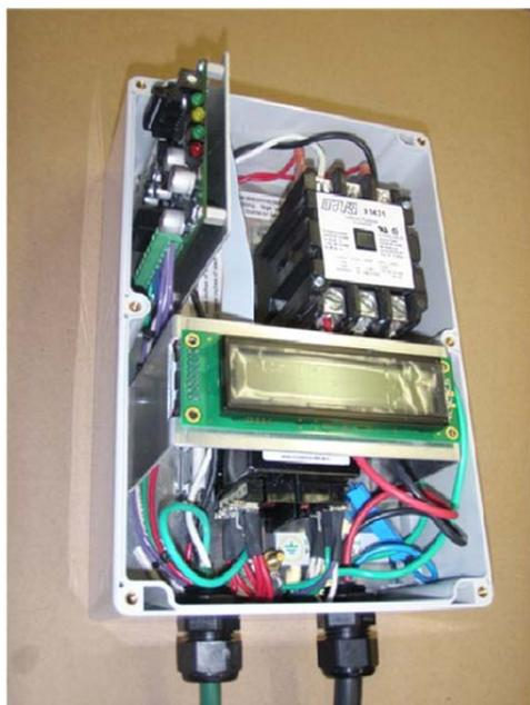
An **Enclosure** is needed for the EVSE. We recommend a polycarbonate box with a clear cover that is UL listed and NEMA 4X rated for water resistance. The clear top allows the LCD or LED to be observed while giving good protection. The box will also be substantial enough to support the cable when it is not in use. There is a requirement for storing the cable when it is not in use and a simple tab and the top of the box will do it.
