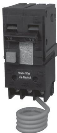
A **GFI Circuit breaker** is needed in your circuit breaker panel. You need to have space to add the breaker in your panel and, you need to have electrical service capacity to you home for the new breaker. The breaker needs to be a 2 pole GFI (ground fault interrupting) breaker for 240 Volt use. The GFI brakes have a white wire coming out the side that must be connected the neutral buss in the breaker box. This will provide the charging current.
