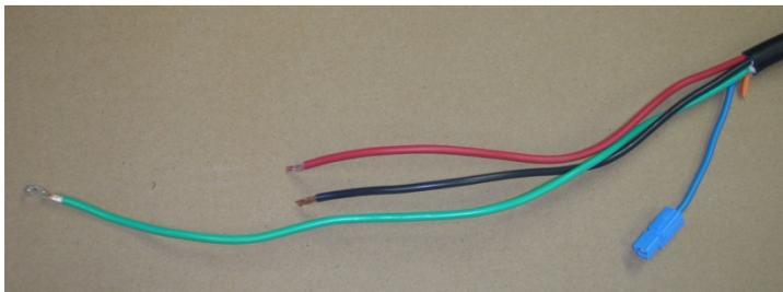
need to be arranged and secured so they disconnect in an orderly fashion. First use an Anderson (plastic blue connector) connector or ¼ inch QD on the pilot wire. Have as little slack as possible, possibly 3 inches so this will pull apart first removing the pilot signal and removing power. Next the two power leads to the J1772
